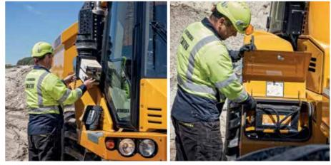
Drain valves make it easier and more controllable to drain oil, as you now have
