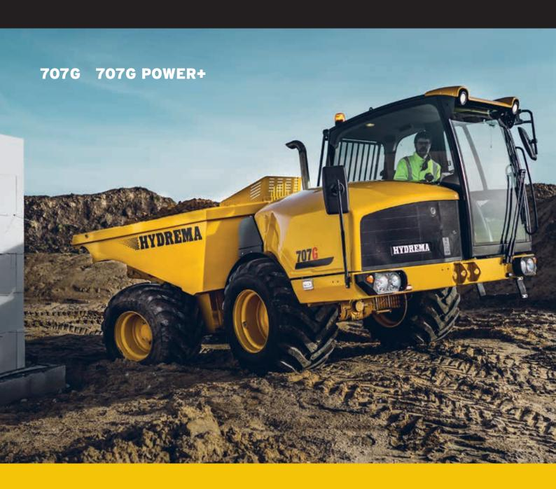
Compact articulated dump truck. Designed with the safety features of a big truck. With a front facing cab, pivot steer & a hydrostatic transmission.
