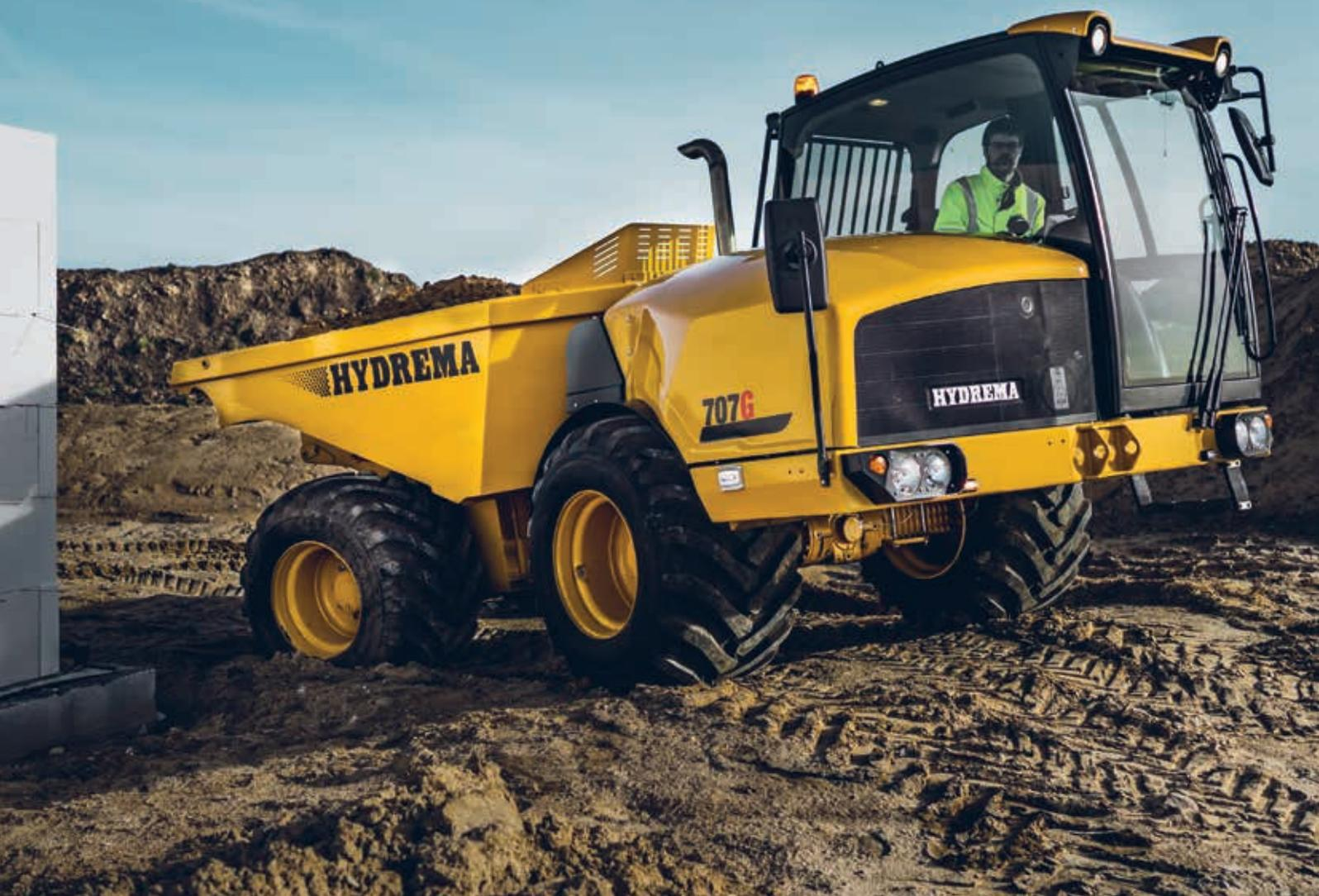
Compact articulated dump truck. Designed with the safety features of a big truck. With a front facing cab, pivot steer & a hydrostatic transmission.
